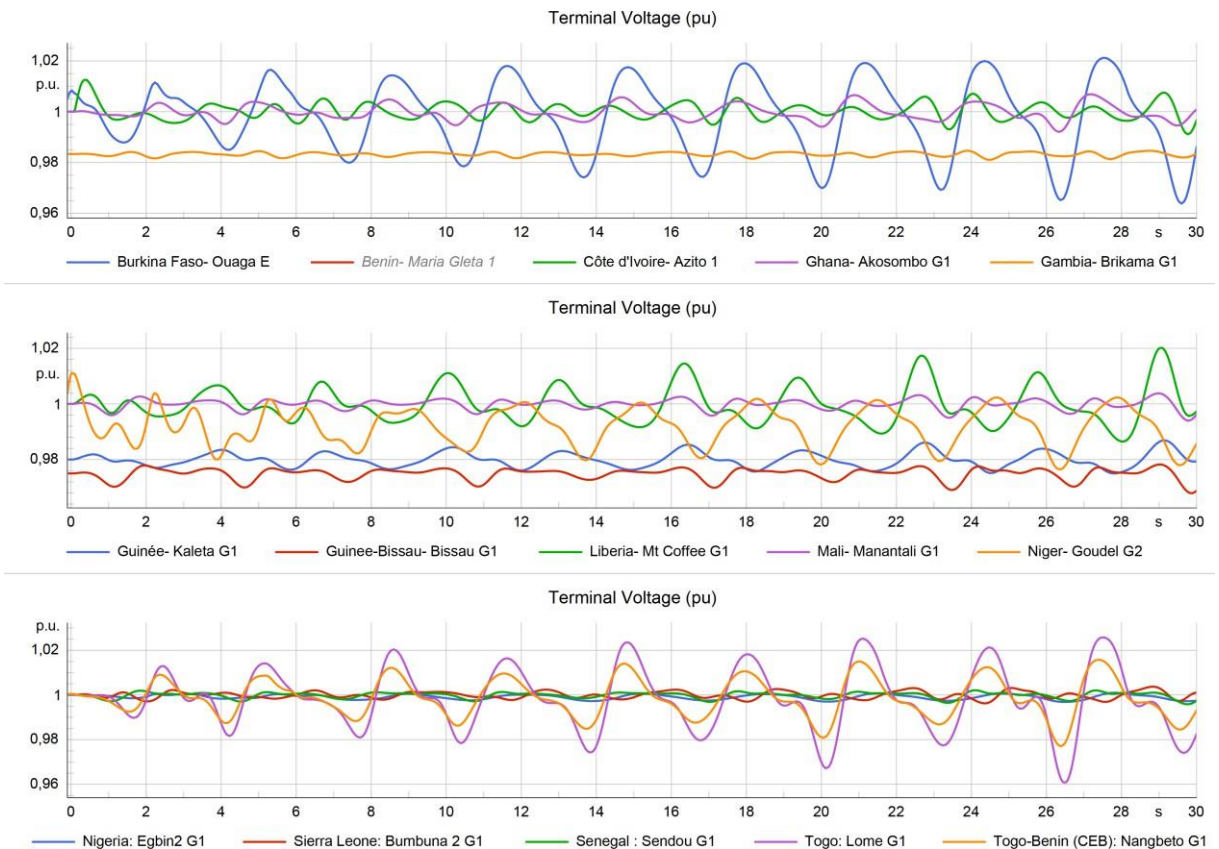
Figure 29 : Evening Voltages, GT trips at CIPREL5 390 MW (Côte d'Ivoire), short list of controlling PP
